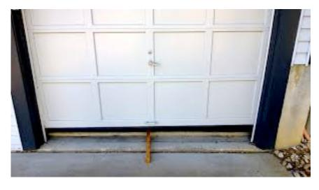
placing a 2×4 on the ground where the door would close. It should reverse after a second or so when the door hits the wood. Also test the photoelectric sensors if you have them by placing something in front of them (not your body). If the door doesn't immediately go back up, you have a problem.
